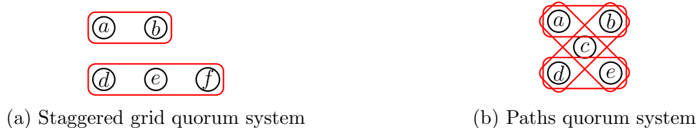
Figure 4.10: The read quorums of the staggered grid and paths quorum systems. The optimal set of complementary write quorums is chosen automatically.
