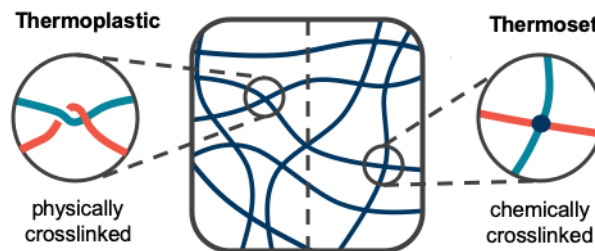
Figure 1.4 Schematic of polymer network showing contrast between physical crosslinks of thermoplastics (left) and chemical crosslinks of thermosets (right).
