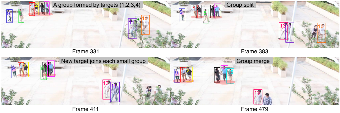
Figure 2.11: Examples of tracking results of our approach on UNIV dataset. Using only the grouping model, we correctly tracked targets (1, 2, 3, 4) in situations where the group split and merge occur. The same color indicates the same target, best viewed in color.
