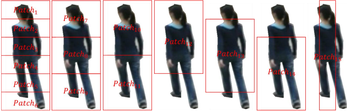
Figure 4.4: Local patches with various scales are defined at different locations of a detection. Patches 1 to 6 have the same size and are served as basic patches, patches 7 to 14 are different combinations of basic patches, and patch 15 captures the middle third region of a detection.
