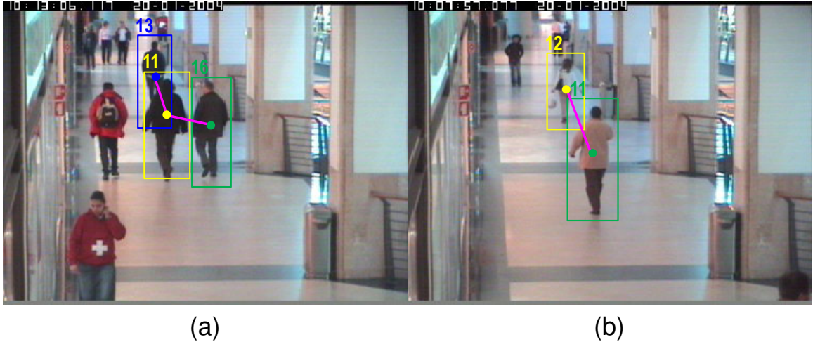
Figure 2.4: Examples of generating incorrect elementary groups if the distances are not normalized.
