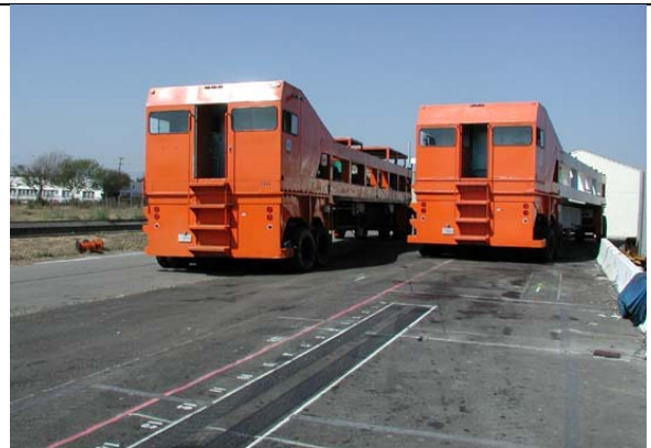
HVS 1 and 2 on modified binder test section, RFS, 2003.
