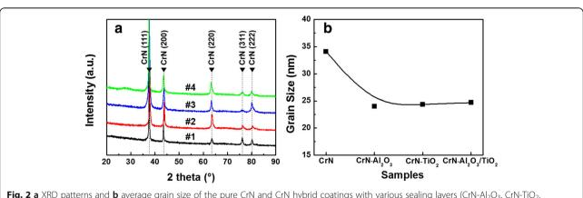
Fig. 2 a XRD patterns and **b** average grain size of the pure CrN and CrN hybrid coatings with various sealing layers (CrN-Al<sub>2</sub>O<sub>3</sub>, CrN-TiO<sub>2</sub>, and CrN-Al<sub>2</sub>O<sub>3</sub>/TiO<sub>2</sub>)
