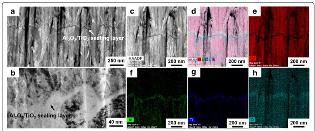
**Fig. 4** TEM/HRTEM/EDX analysis of the typical CrN-Al<sub>2</sub>O<sub>3</sub>/TiO<sub>2</sub> hybrid coating: **a** low magnification bright field image. **b** HRTEM image of the nanolaminate-Al<sub>2</sub>O<sub>3</sub>/TiO<sub>2</sub> sealing layer. **c-h** EDX mapping results of Cr, Al, Ti and O elements
