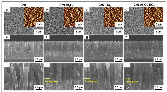
Fig. 3 SEM surface images and cross-sectional images of the pure CrN and CrN hybrid coatings with various sealing layers. **a, e, i** CrN. **b, f, j** CrN-Al<sub>2</sub>O<sub>3</sub>. **c, g, k** CrN-TiO<sub>2</sub>. **d, h, I** CrN-Al<sub>2</sub>O<sub>3</sub>. **c**, **c**, **d, h, I** CrN-Al<sub>2</sub>O<sub>3</sub>. **c** (a) TiO<sub>2</sub>. The corresponding AFM images were inserted in Fig. 3a–d
