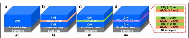
**Fig. 1** Schematic illustrations of the cross-sectional structure. **a** Pure CrN coating. **b** CrN-Al<sub>2</sub>O<sub>3</sub>; CrN coating with a 20 nm Al<sub>2</sub>O<sub>3</sub> sealing layer. **c** CrN-TiO<sub>2</sub>; CrN coating with a 20 nm TiO<sub>2</sub> sealing layer and **d** CrN-Al<sub>2</sub>O<sub>3</sub>/TiO<sub>2</sub>; CrN coating with a 20 nm nanolaminate-Al<sub>2</sub>O<sub>3</sub>/TiO<sub>2</sub> sealing layer.
