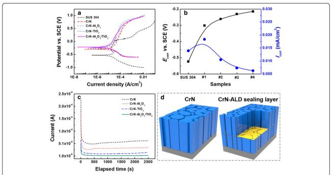
**Fig. 5** Potentiodynamic and potentiostatic curves of the SUS304 substrate, SUS304 substrate coated with CrN, CrN-Al<sub>2</sub>O<sub>3</sub>, CrN-TiO<sub>2</sub> and CrN-Al<sub>2</sub>O<sub>3</sub>/TiO<sub>2</sub> in 3.5 wt. % NaCl solution: **a** potentiodynamic curves. **b** calculation value of the corrosion potential and corrosion current density. **c** potentiostatic curves. **d** schematic illustration of corrosion behavior of the pure CrN coating and hybrid coating
