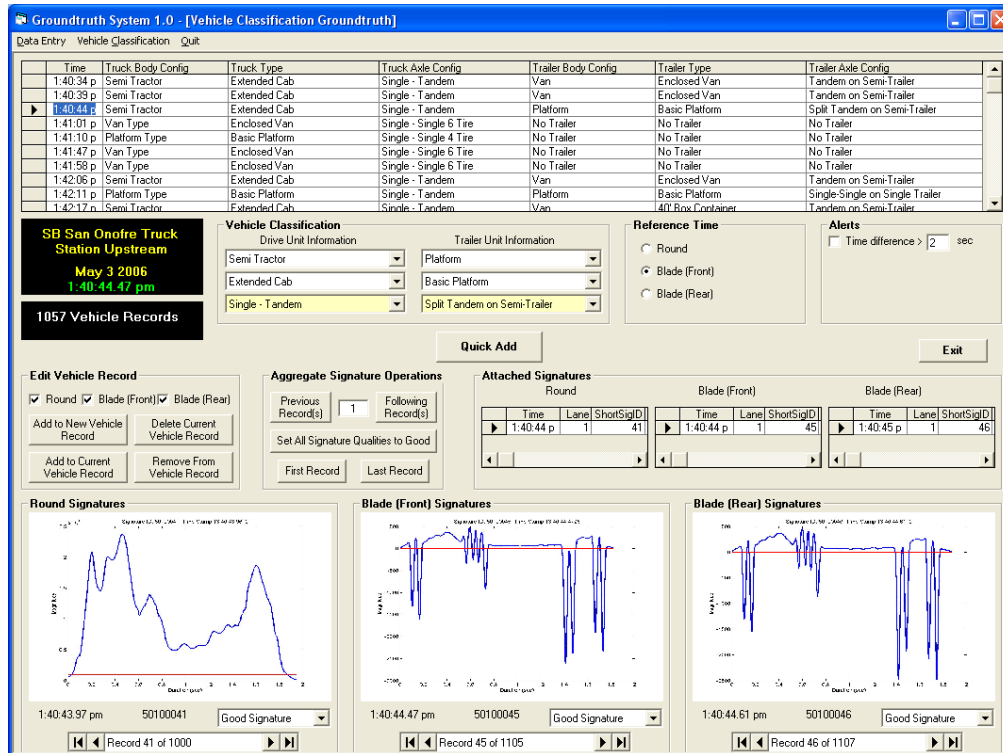
Figure 3.5. Commercial vehicle classification groundtruth data entry system
