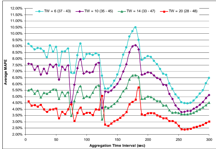
Figure 7.8 MAPE for travel time estimation for square/square loops case
