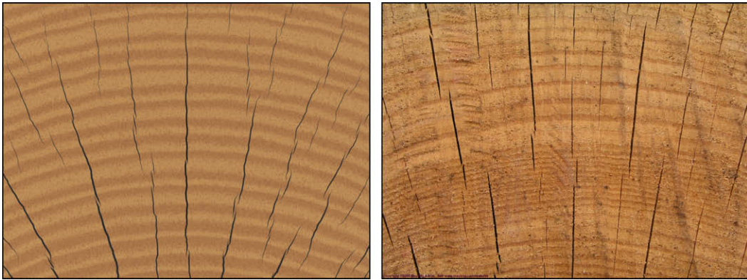
Fig. 8. We show an example of wood cracking perpendicular to the grain at the sawn end of a tree trunk ( left ) compared to a photograph ( right , copyright 2005 Mayang Adnin). We used a concentric stress field, radiating outward from the center of the tree point, to model the anisotropic stress. Total computation time was 10.1 min on a 79,202 element mesh.
