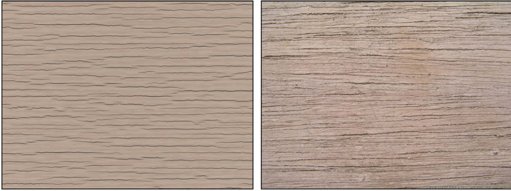
Fig. 7. An example of cracked wood along the grain ( left ) compared to a photograph ( right , copyright 2006 Mayang Adnin). We used a vertical stress field to model the anisotropic material. Total computation time was 19.2 min on a 79,202 element mesh.
