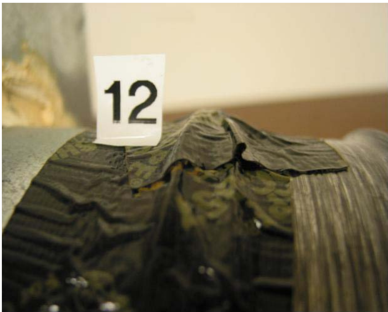
Figure A14. Sample 12. The end of the tape has wrinkled and shrunk.
