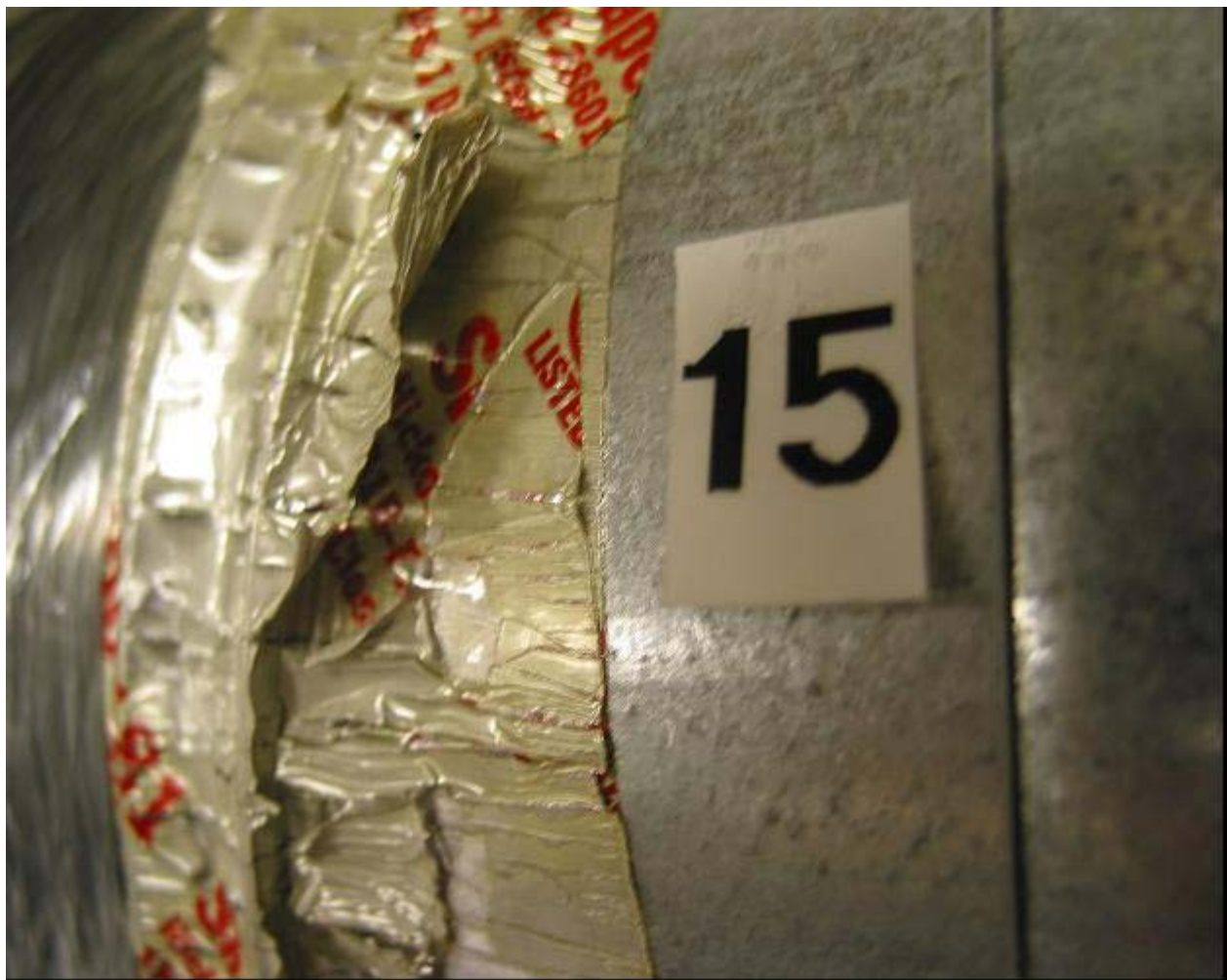
Figure A18. Sample 15. Like samples 13 and 14, this sample is also peeling and cracking. This figure shows how the metallized layer is splitting from the adhesive layer.
