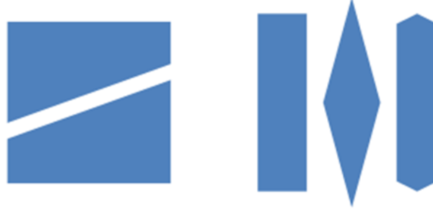
Figure 2.4: Unit cell examples. A square unit cell with a slit is shown on the left. Three different unit cells with two symmetry planes are shown on the right.
