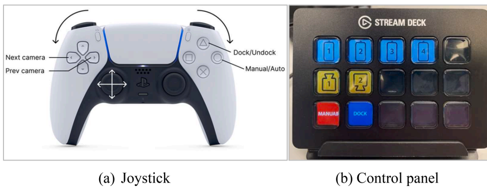
Fig. 10. Joystick and the control panel for steering autonomous ferry(s) in the experiment (c.f. Hanssen (2022)).
