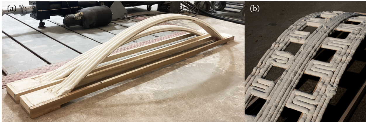
Figure 5.5: To test the concept of conformal 3D printing on a bending-active formwork, a series of small-scale experiments were conducted. (a) shows configurations with one strip, while (b) demonstrates a configuration with a grid of multiple strips.
