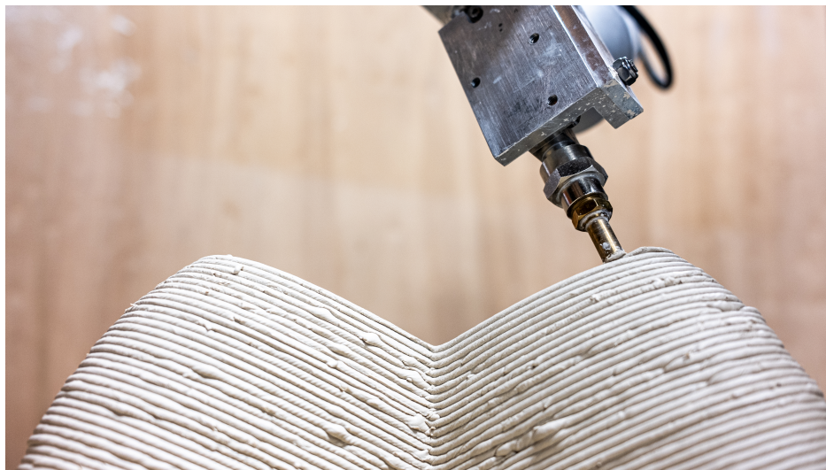
Figure 7.10: Multi-axis extrusion and conformal nozzle orientation that follows the tangent vector of the base surface.
