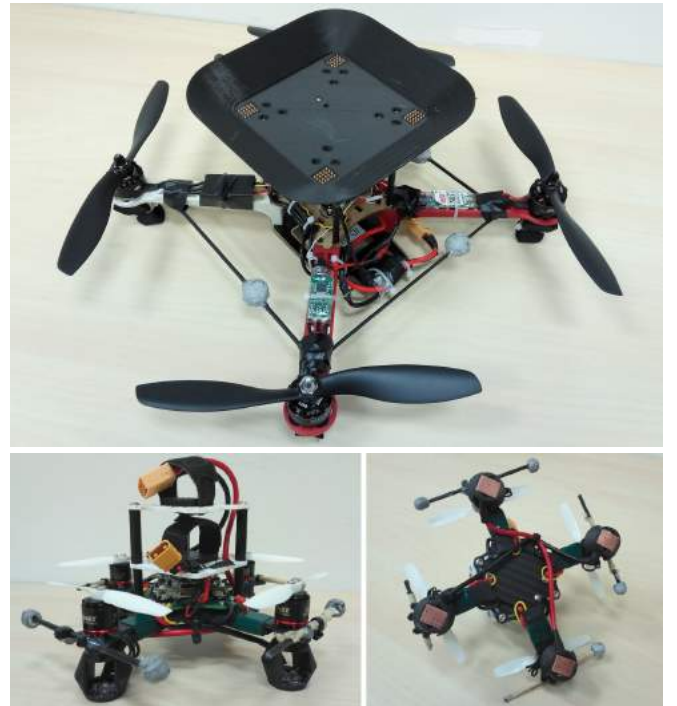
Fig. 3: Top: Main quadcopter with the docking platform and spring loaded connectors. Bottom: Flying battery with the docking legs and copper plate connectors.
