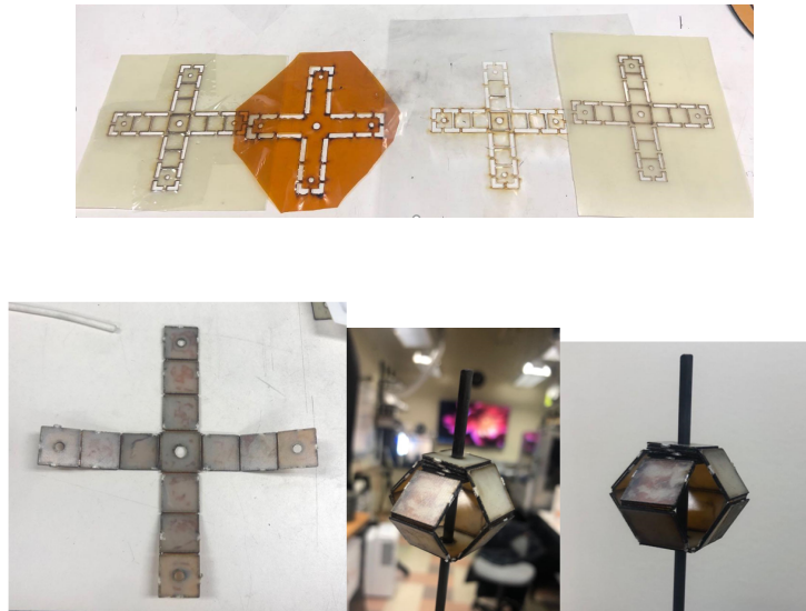
Figure 3.12: Fabrication of the Sarrus linkage
