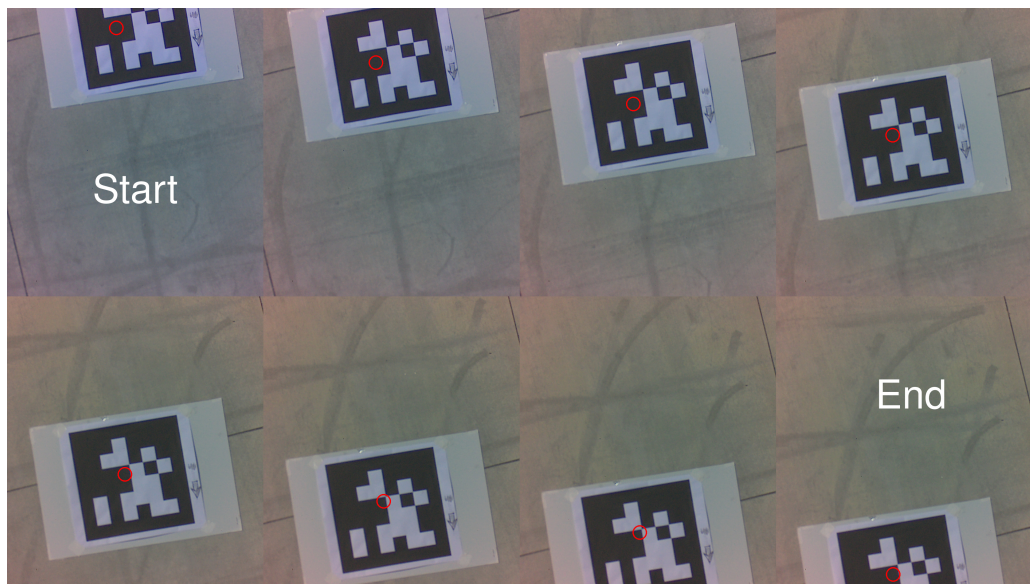
Figure 5.11: The figure illustrates the targeting precision of BANNERS during a simplified test scenario. The circular target accurately traces the center of the April tag throughout a primarily linear translation motion.
