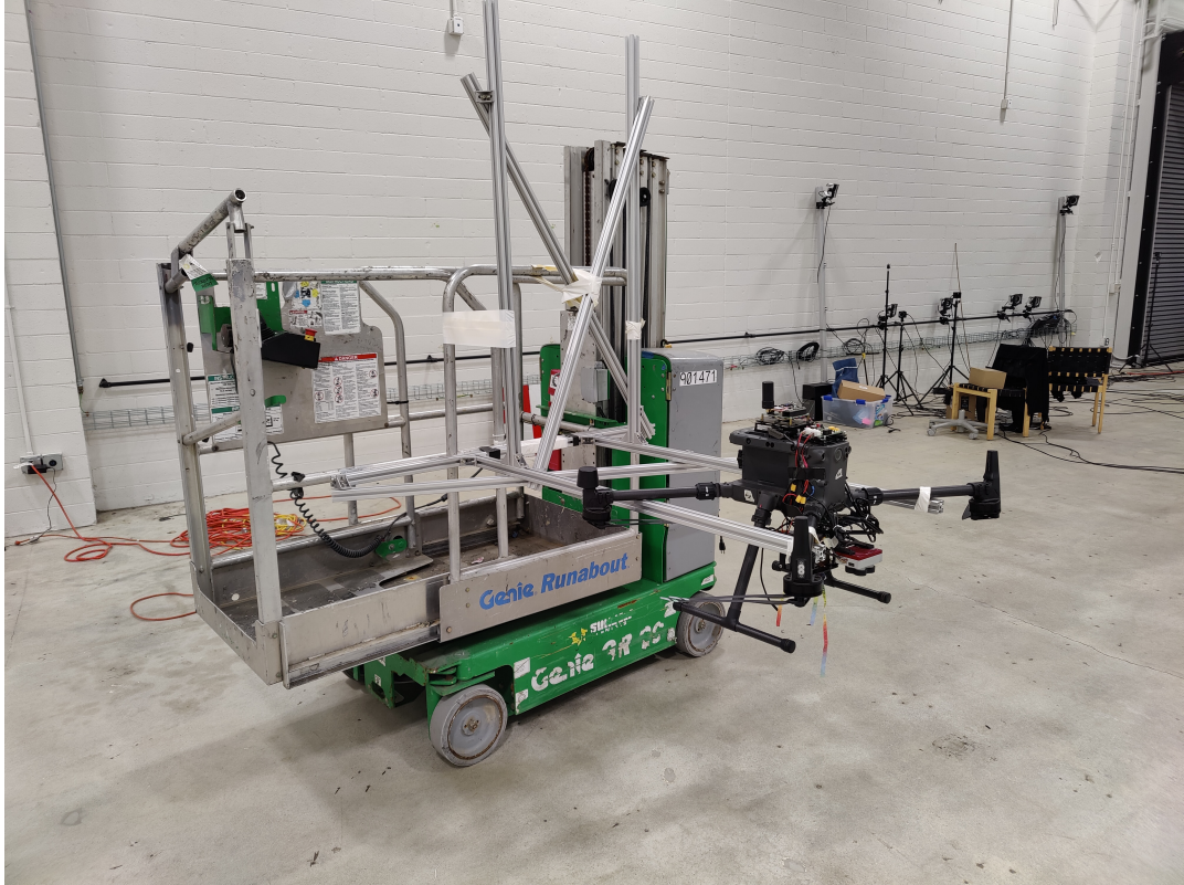
Figure 5.10: The provided image showcases the test rig employed to comprehensively simulate the flight of ASTRO, serving purposes such as calibration and debugging. ASTRO is securely affixed to the side of the mast lift, enabling it to be maneuvered in close proximity to a designated target, thereby facilitating the collection of consistent and reliable data.
