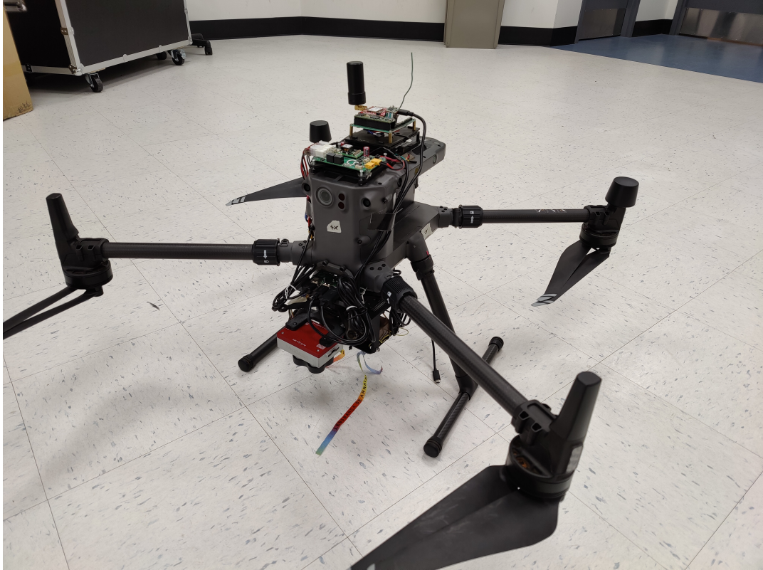
Figure 4.3: ASTRO: The data collection robot showcasing the integration of DJI Matrice M300 platform. The "roof" section is home to the exposed power and data connections, accompanied by the DJI manifold system facilitating power and data transfer from the UAV. Notably, the high precision GNSS system is also positioned on the roof, enhancing geo-referencing capabilities.
