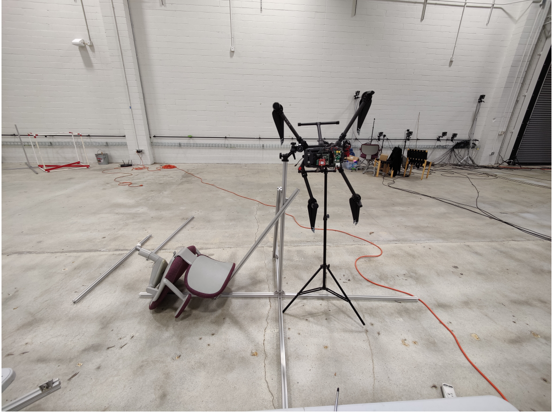
Figure 5.1: This test was part of confirming the camera intrinsics estimates from Kalibr. The robot is held rigidly within a well defined coordinate frame to remove run to run variance. PNP was then used to solve for the pose of the drone given well defined world points as reference. The mount also allowed us to confirm the pose estimated by PNP by making the pose of the drone obvious.
