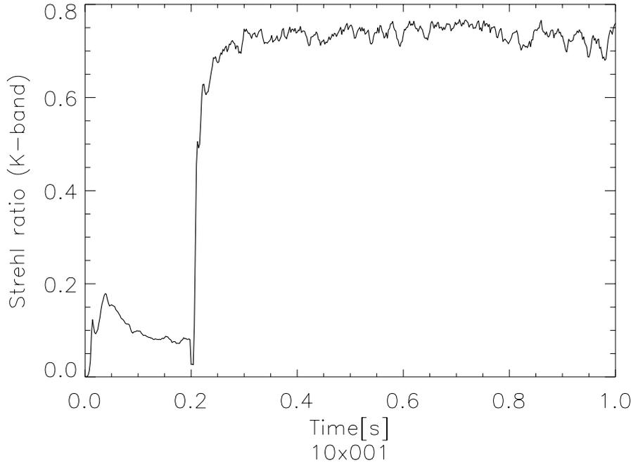
Figure 4: Time series of the AO loop closing in presence of scalloping (here, starting with  $10 \times 001$ ). This is the Short exposure K-band Strehl ratio, the Long Exposure Strehl at 1.0s is  $\sim 70.56\%$ .
