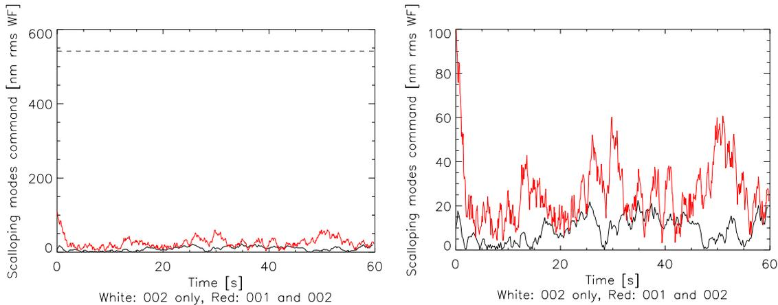
Figure 5: Scalloping residuals as a function of time (in nm rms). The dashed line shows the original input value. Black line is when only  $10 \times 002$  is sent at the beginning and only mode 002 is corrected (other mode has a gain of zero). The red curve is when  $10 \times 001 - 10 \times 002$  is introduced and both modes corrected. On the right, is a zoom of the same curve as on the left.
