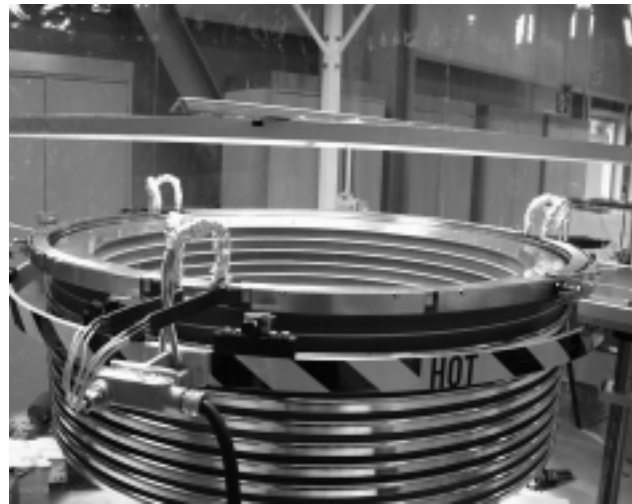
Figure 3 - Installation of Field Shapers
