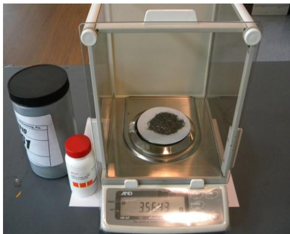
Figure 7.1: Determining the weight of the utilized materials – natural graphite and sodium cholate.
