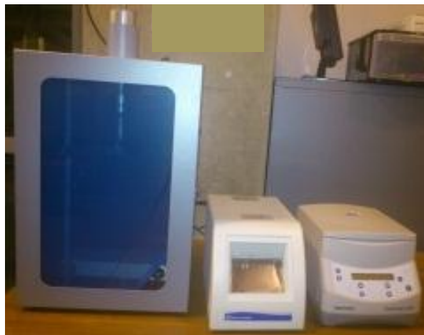
Figure 7.2: Photograph of ultrasonication (Fisher Scientific Model 750 Sonic Dismembrator) and centrifuge (Fisher Scientific Eppendorf 5424 Microcentrifuges) equipment at Nano device laboratory, UCR.
