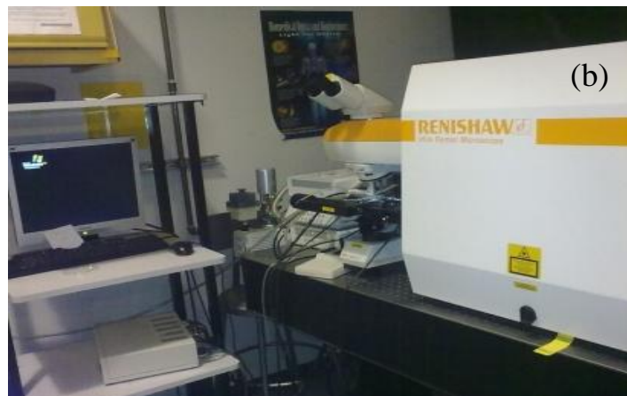
Figure 4.7: (a) Renishaw Raman microscope system used for Raman measurement. (b) Photograph of the Raman instrumentation system in the Nano device laboratory, UCR.
