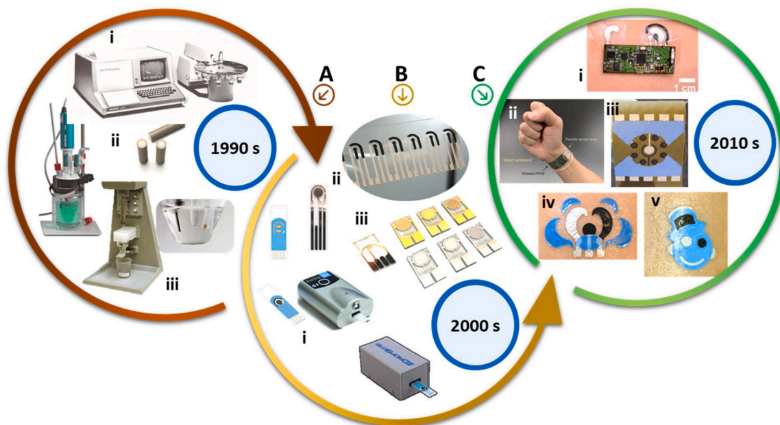
Fig. 1. Evolution of electrochemical analyses: (A) Classical benchtop instrument based analytical devices in 1990s: (i) Benchtop electrochemical analyzer with the conventional electrochemical cell setup [21], (ii) electroanalytical cell setup with rotating disc electrodes for analyses (Web-source: https://www.metrohm-autolab.com/ ), (iii) dropping mercury based electroanalytical cell system (Web-source: http://www.princetonappliedresearch.com ); (B) Handheld systems for onsite electroanalyses in 2000s: (i) the portable hand-held palm-sized analyzers (Web-source: https://www.palmsens.com ), (ii) the commercial screen printed electrode systems for onsite analyses in small sample amounts (Web-source: http://www.dropsens.com ), (iii) screen printed electrodes with the flexible substrate, (iii) photolithographic electrode system for ultra-trace analysis (Web-source: https://www.micruxfluidic.com/ ); (C) Skin-worn tattoo / patch / textile based wearable biosensors in 2010s: (i) tattoo based wearable sensor for alcohol detection [22], (ii) wearable patch “Smart wristband” for multi-analyte detection [2], (iii) textiles based wearable system for detecting multiple analytes [51], (iv) printed temporary transfer tattoo epidermal electrochemical sensors [33], (v) the tattoo based “smiling” wearable for sweat pH sensing [32].
