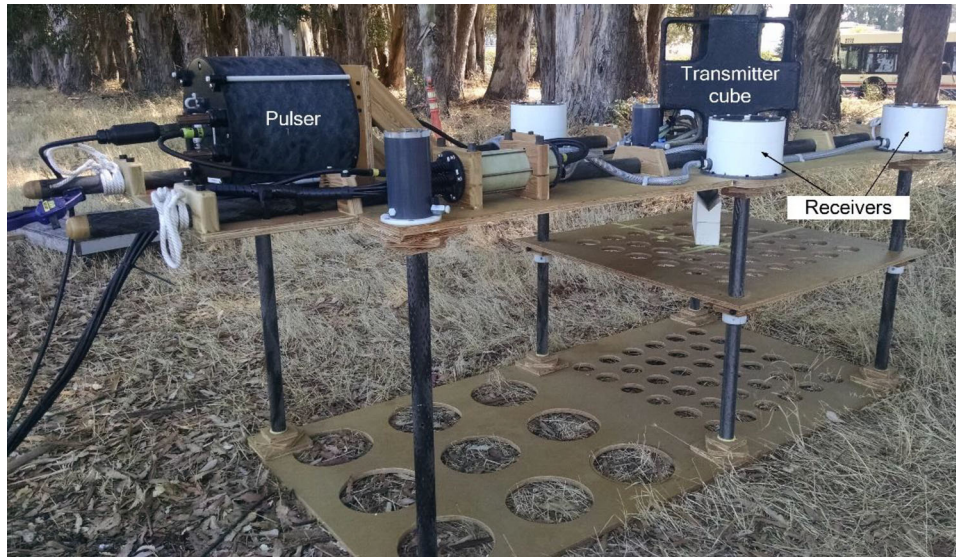
FIGURE 2 Marine system for a cued mode operation during land testing.
