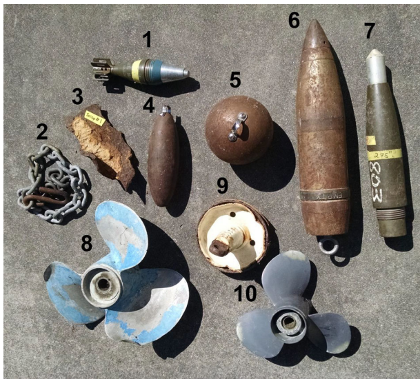
FIGURE 5 Objects used for system testing: (1) 60-mm mortar, (2) chain, (3) a piece of scrap metal, (4) 230-mm spheroid, (5) 152-mm shotput, (6) 105-mm projectile, (7) 70-mm rocket, (8) large propeller, (9) anchor and (10) small propeller.
