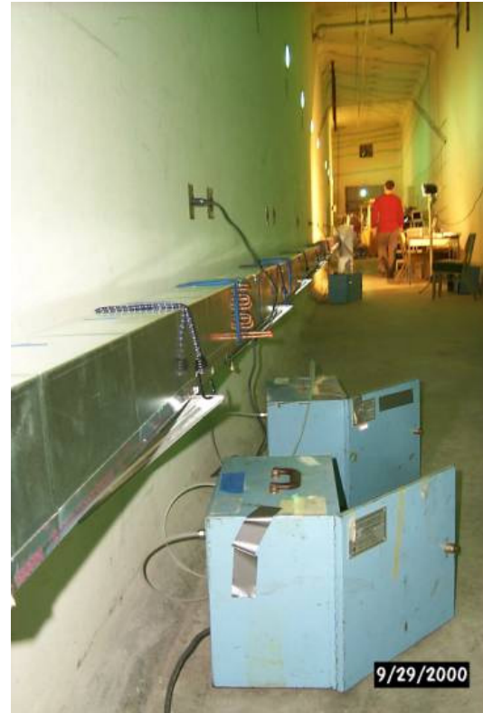
Figure 7. Illustration of Coil Fouling Apparatus showing the Duct and Particle Samplers
