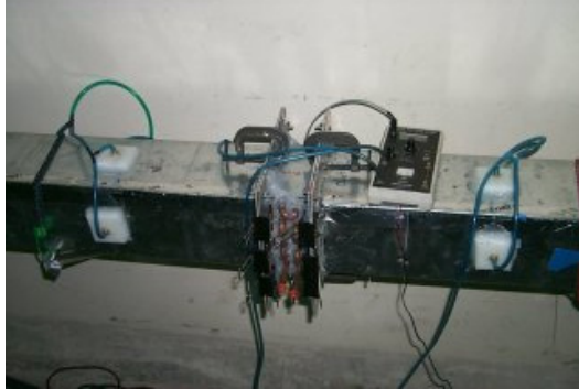
Figure 8. Measurement of the coil pressure drop
