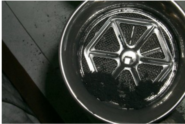
Figure D4. Dust remaining inside of the sifter
