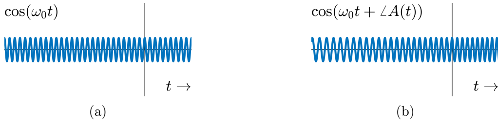
Figure 2-6: Phase variations in an ultrafast pulse: Figure 2-6a plots the same information as that in Fig. 2-5c. That is, we have plotted the fluctuations that arise from the carrier term alone. In 2-6b we see variations in the phase, caused by the phase of the envelope A(t) . These variations modulate the regular fluctuations of the carrier. Thus, 2-6b is a representation of the total phase of E(t) , whereas 2-6a is a representation of the phase of the carrier alone.
