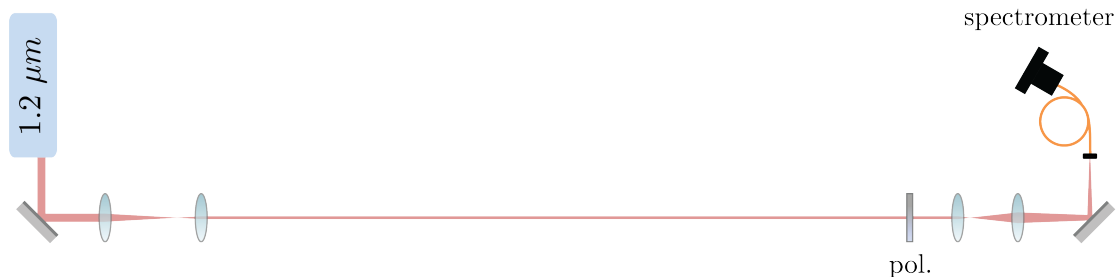
Figure 4-2: Direct-path layout: Compared to the complete layout in Fig. 4-1, all mirror flip-mounts were in the down position, and we removed the nonlinear crystal and bandpass filter. The latter two elements were reinserted for the measurement of the SHG spectrum.
