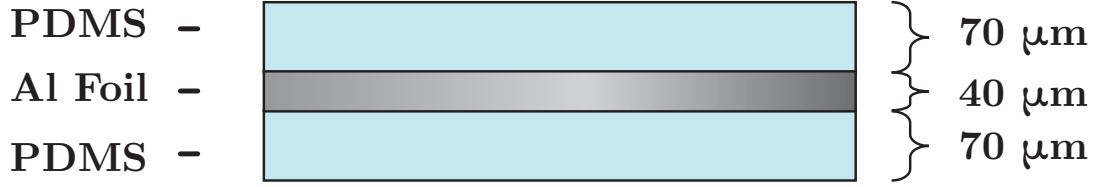
Figure C.5: Illustration of the PDMS/Al hybrid membrane sandwich.
