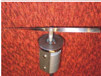
Figure 2. The mixing fan, with blades folded for insertion in the duct (top) and with blades unfolded
