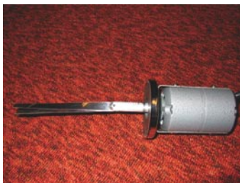
Figure 1. The whip injector; note the small, light weight CO 2 cylinder
