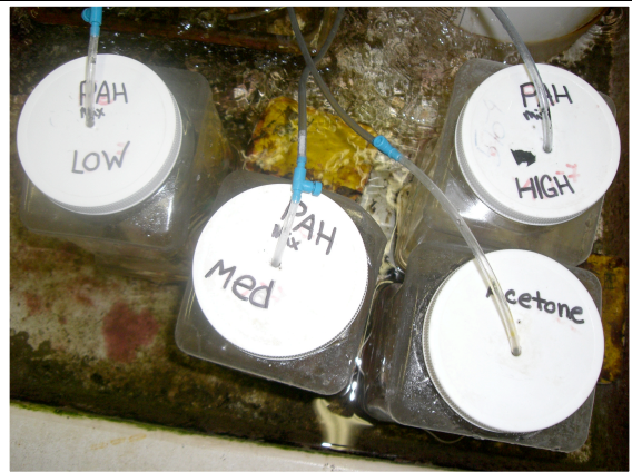
Figure 7. Experimental setup with 4 aquaria in which brittlestars were exposed to low, medium and high PAH concentrations, with Acetone exposure as the control.
