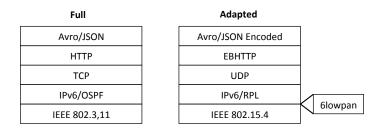
Figure 4.18: Layers in the protocol stack, and the protocols in use in the full version of sMAP, next to the version adapted for embedded devices.
