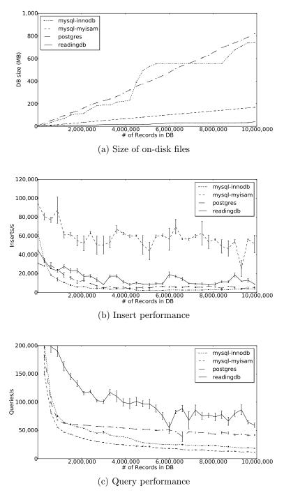
Figure 5.7: readingdb time series performance compared to two relational databases. Compression keeps disk I/O to a minimum, while bucketing prevents updating the B+-tree indexes on the time dimension from becoming a bottleneck. Keeping data sorted by stream ID and timestamp preserves locality for range queries.
