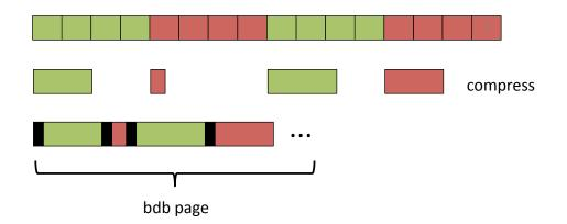
Figure 5.2: The **readingdb** historian first buckets data along the time axis to reduce the index size, storing values near other values with neighboring timestamps from the same stream. It then applies a run-length code followed by a Huffman tree to each bucket, resulting in excellent compression for for many commonly-seen patterns.
