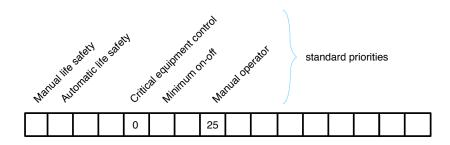
Figure 2.5: An example state of a BACnet priority array. In this case, the present value for this controller would take on the value 0 since that is the highest-priority, non-null value present.
