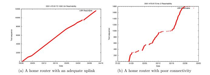
Figure 4.1: The results of five-minute external connectivity tests over a period of weeks for two residential deployments. A connection with no problems would be shown as a straight line.
