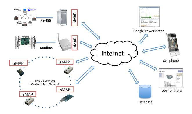
Figure 4.13: Part of the sMAP ecosystem. Many different sources of data send data through the Internet to a variety of recipients, including dashboards, repositories, and controllers.
