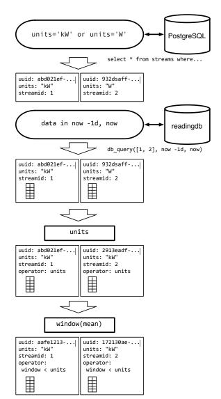
Figure 7.2: The complete pipeline needed to execute our example query. The language runtime first looks up the relevant time series using the where-clause, and uses the result to load the underlying data from **readingdb**, using the data-clause. It then instantiates the operator pipeline, which first converts units to a consistent base and then applies a windowing operator.
