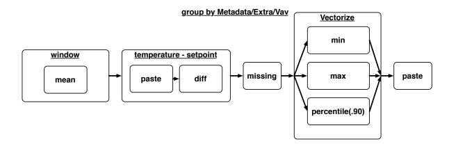
Figure 7.13: The execution pipeline for the query shown in Figure 7.12. The group-by clause exposes the fundamental parallelism of this query since the pipeline is executed once per distinct location.
