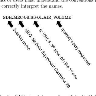
Figure 2.6: An example of a BACnet point name from Sutardja Dai Hall, on the Berkeley campus. In this case, the point name includes both spatial (building, floor, and zone) information, network information (the controllers' address), and functional information (air volume). Interpreting this requires knowing the convention in use.
