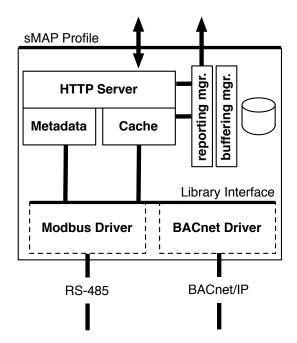
Figure 4.10: Our implementation of sMAP provides a clean runtime interface against which to write reusable "driver" components, which contain logic specific to the underlying system. The runtime is responsible for formatting sMAP objects, implementing the resource-oriented interface over HTTP, and managing on-disk buffering of outgoing data. It also provides configuration-management and logging facilities to users.
