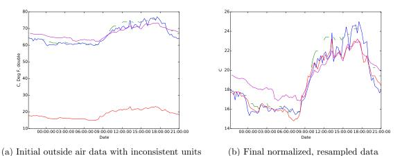
Figure 7.11: The application interface lets us quickly resample and normalize raw data series.
