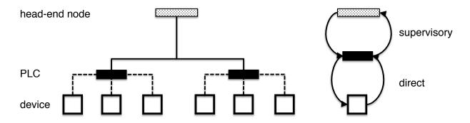
Figure 2.3: The two-level architecture of many existing building separations, with a logical and physical distinction between direct and physical control. This is shared with a typical Supervisory Control and Data Acquisition (SCADA) system.
