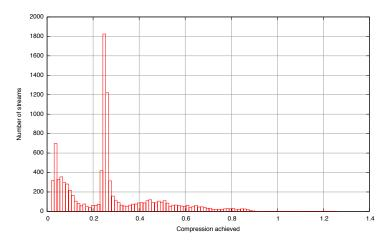
Figure 5.5: Compression achieved across all streams in the time series store at a point in time. A significant number of streams are either constant or slowly changing, which result in 95% or greater compression ratios. The spike in streams which are compressed to about 25% are plug-load meters which noise making them difficult to compress.
