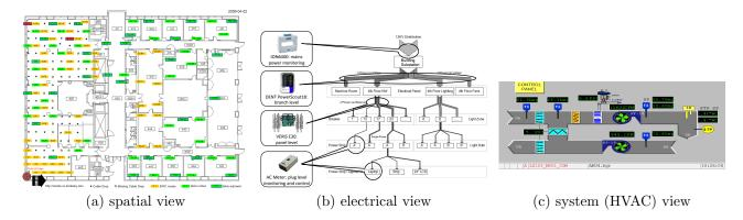
Figure 3.3: Multiple different views of the relationships between system components exist and interact in physical space. The HAL allows applications to be written in terms of these relationships rather than low-level point names.
