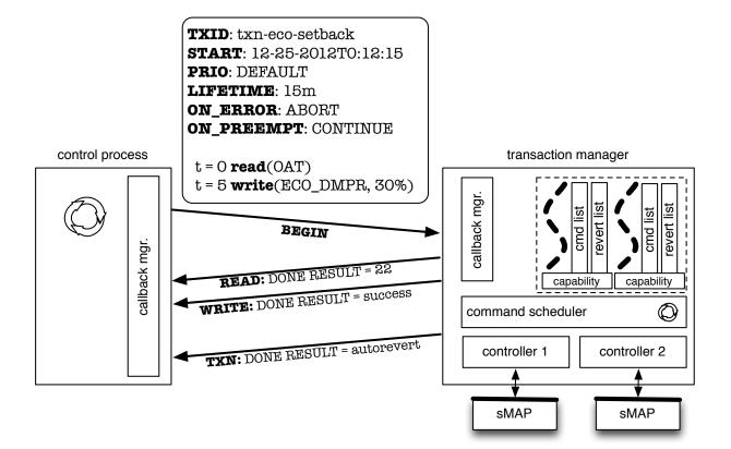
Figure 8.2: A transaction manager (TM) communicating with a remote Control Process. The TM prioritizes requests from multiple processes, alerting the appropriate control process when necessary. The TM also manages the concurrency of the underlying physical resources, and provides all-or-nothing semantics for distributed actions. It provides the ability to roll back a running transaction.
