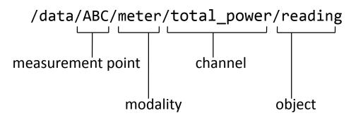
Figure 4.3: Canonical sMAP URL for the "total power" meter of a three-phase electric meter.
