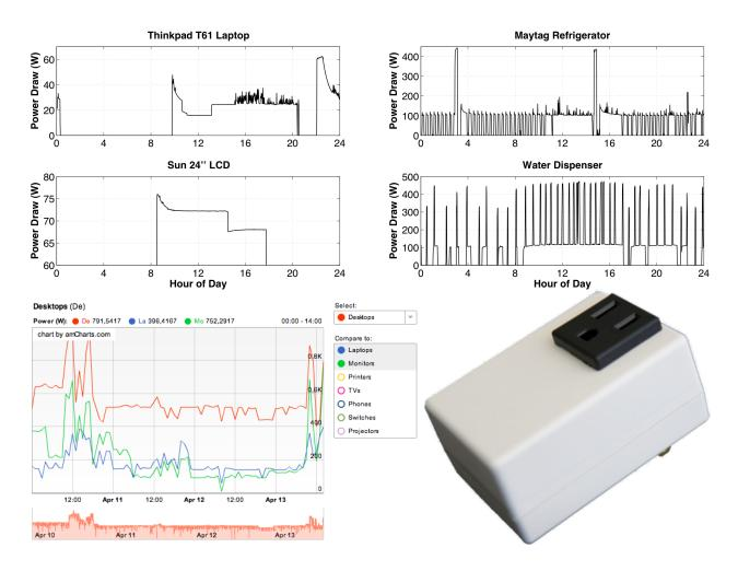
Figure 4.17: ACme wireless plug-load meters (bottom right) are used to monitor power consumption of various appliances, including a laptop and a LCD display in the top left, a refrigerator and a water dispenser in the top right, and aggregate consumptions in bottom left.
