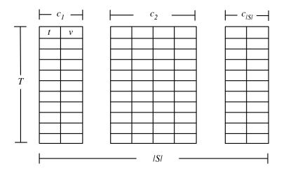
Figure 6.1: Each time series being processed is a matrix with a notionally-infinite height (each row shares a time stamp), and a width of  $c_i$ , representing the number of instrument channels present in that series. Sets of these may be processed together, forming the set S of streams.
