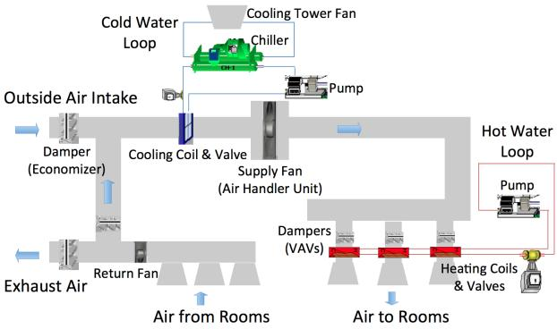
Figure 2.1: A typical process diagram of an HVAC system loop in a commercial building.
