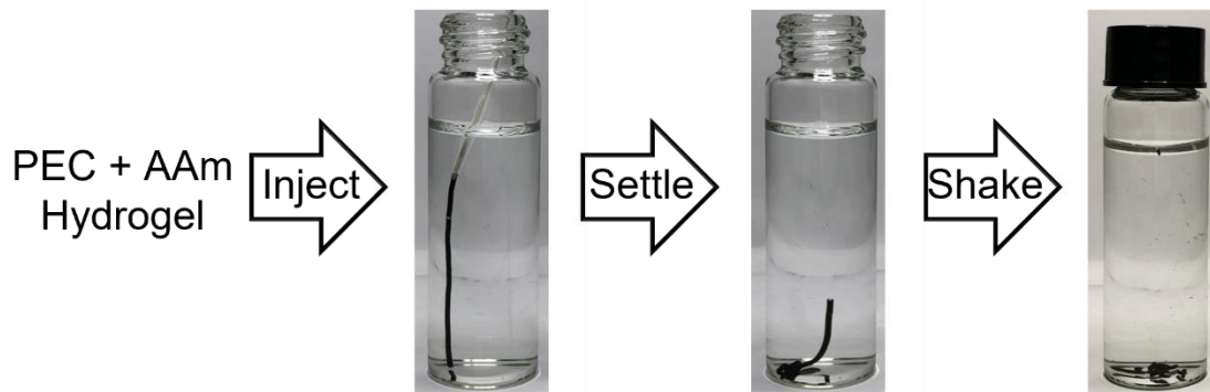
Figure 4-S7. Photos showing injectability and interim insolubility of PEC+AAm hydrogel in an aqueous environment.
