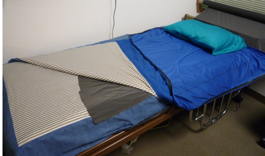
Figure 4.1: The pressure sensitive bedsheets setup with sensing eTextile layers.
