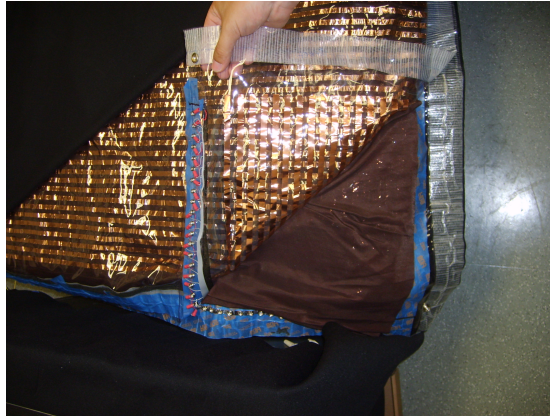
Figure 2.1: The structure of textile sensor and sensor array design
