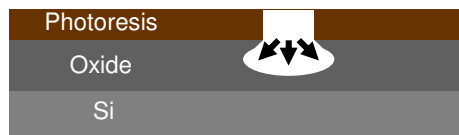
Figure 2-12 – Undercutting due to over etching of oxide layer
