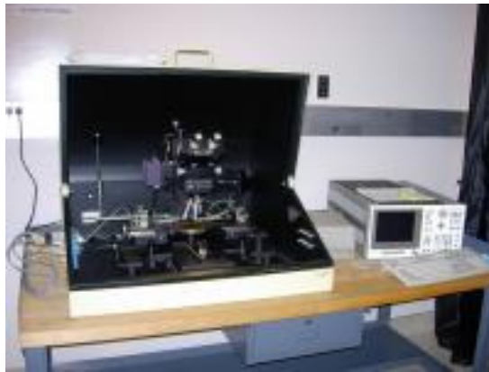
Figure 3-8 – HP Parametric workstation connected to a Hewlett-Packard 4155A Semiconductor Parameter Analyzer
