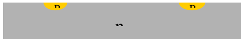
Figure 2-4 - bare n-type silicon with p++ doped source and drain (yellow) after etching oxide layer with 10% HF solution
