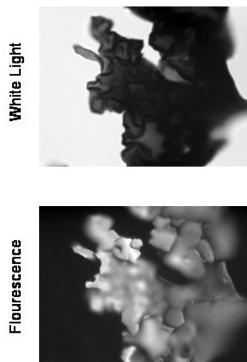
Figure 4-14 – Image of polythiophene-3-boronic acid (top) and fluorescence image after exposure to Alizarin Red S (bottom).
