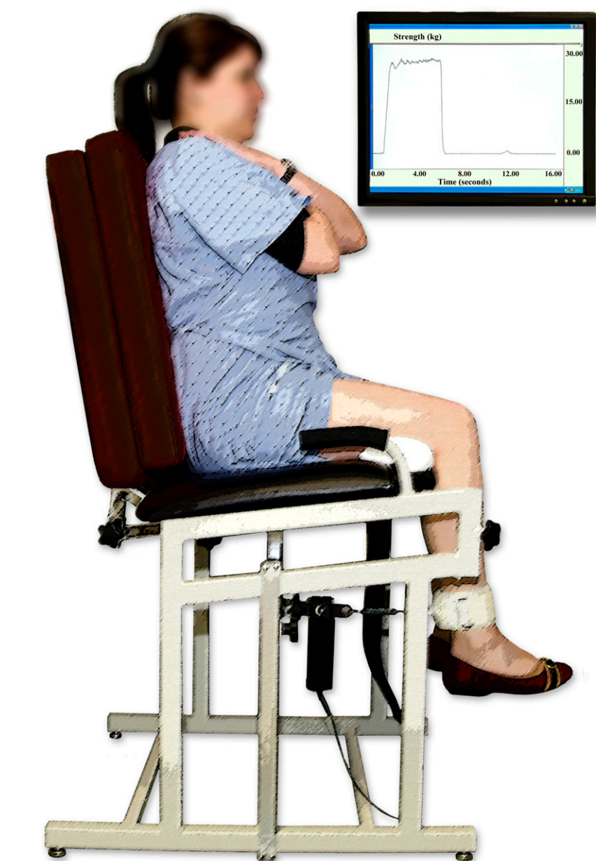
Figure 4. Standard operating procedure for isometric quadriceps strength assessment. During the maneuver, vigorous encouragement of the patient is needed. Patient is positioned in a standardized fashion (typically sitting with knees and hips in 90° flexion or, less often, supine [248]). Maximal voluntary contraction force (reported in kilograms or newtons) can be reliably assessed as the best of three reproducible maneuvers. Maximal voluntary contraction is recorded as the maximal force that can be maintained for 1 full second.
