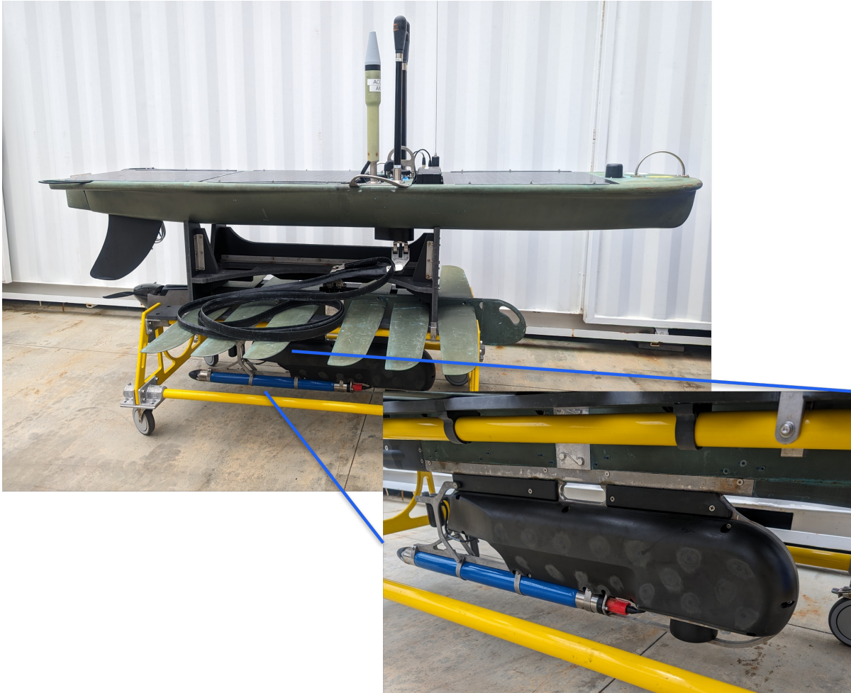
Figure 1.2. The Wave Glider is seen prepped for deployment. Top component is the float, and the sub is beneath it attached to an umbilical (not pictured). The 25 kHz transducer is below the sub component towards the aft rudder and underside of the vehicle. The bottom picture is a zoom-in on the sub and transducer
