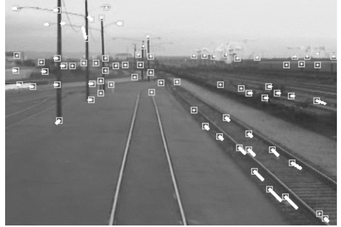
Fig. 3. Detected corner features (square boxes) and their optical flows. Note that the line features can cause false matches (aperture problem). The optical flows were exaggerated 3 times for visibility.
