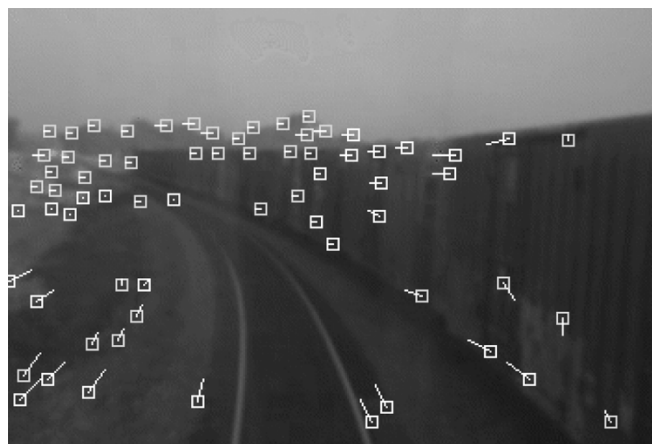
Fig. 8. RANSAC with a seven-point algorithm does not work well. RANSAC's scoring function says that 52 out of 68 correspondences are consistent with the resulting essential matrix, but the reprojection error tells that only 29 are consistent (white boxes).
