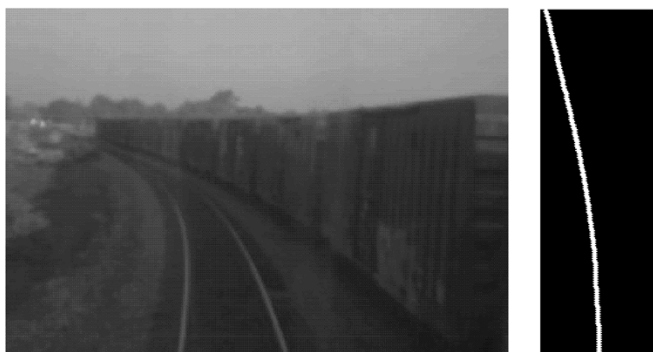
Fig. 7. Example video sequence (first frame) and train trajectory reconstructed from the suggested ego-motion estimation.
