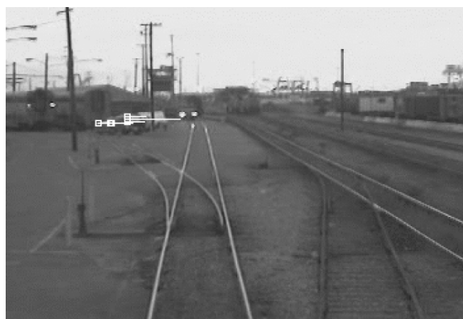
Fig. 9. Detected moving object with the trajectories of its corner features.
