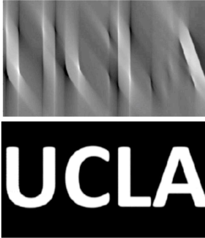
Figure A2-4 Shows that continuously adding projections, as shown in Fig. A2-3, in the object space eventually yields the reconstructed image (top) Reconstructed image by adding projections from [0, 60] degrees. (bottom) Reconstructed image by adding projections from [0, 180] degrees where the object (white UCLA text on black background) is reconstructed accurately.
