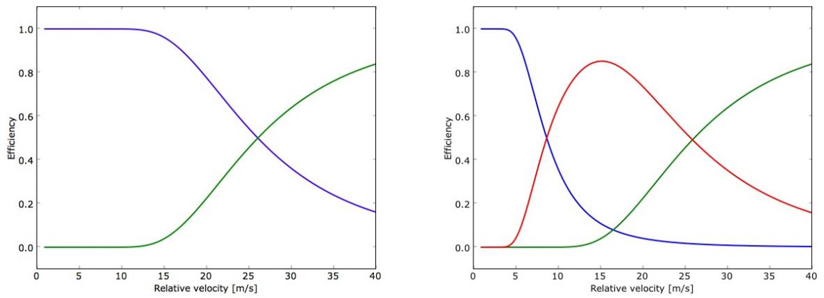
Fig. 3: Coagulation (in green) and fragmentation (in blue) efficiency as a function of relative velocity in the Tail model. On the left, the critical velocities are  $v_f = v_c = 30$  m/s; on the right,  $v_f = 30$  m/s and  $v_c = 10$  m/s, so there is a bouncing region, whose probability is represented by the red line.
