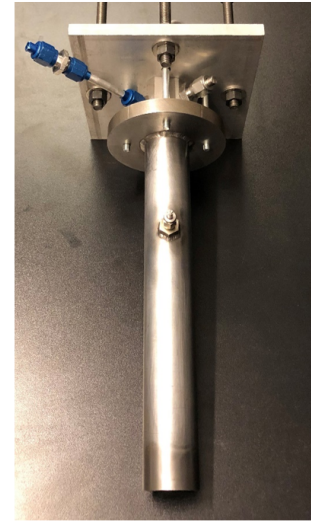
Figure 5.1: ( left ) Cross-sectional view of combustor assembly and ( right ) completed hardware assembly.
