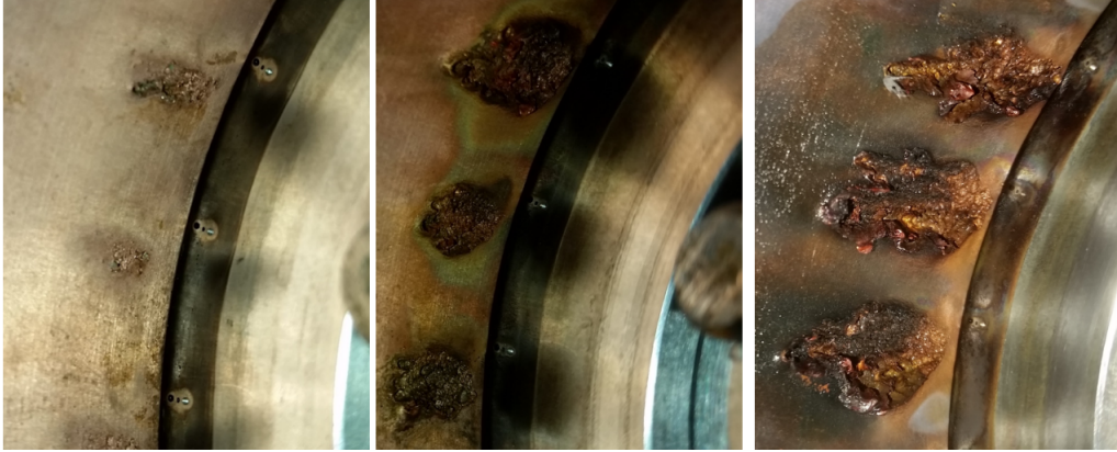
Figure 5.2: Thermal damage in RDE after 4, 8, and 12 hot-fire tests. Burn times lasted less than one second. Borrowed from [42].
