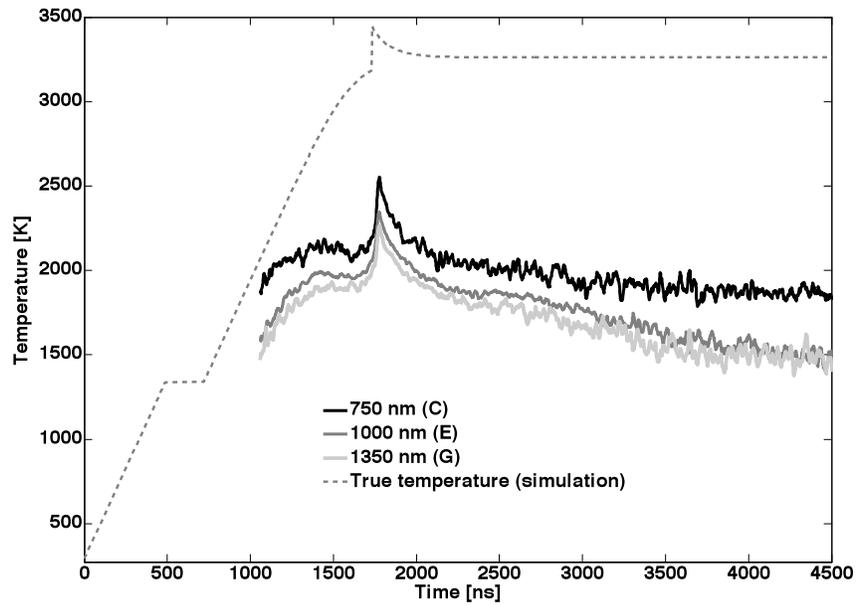
**Figure 3: Brightness temperatures of an ion-beam heated gold target and the corresponding simulation (dashed). The uncompressed part of the beam hits the target at 0 ns, followed by a 2 ns compressed bunch at 1,600 ns.**
