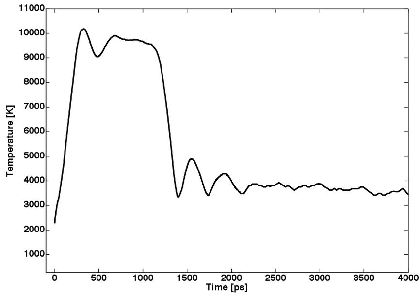
**Figure 4: The brightness temperature at 1000 nm of a laser-beam heated copper target. The 100 fs laser pulse arrives at 0 ps. The “ringing” of the signal is instrumental and caused by the limited frequency bandwidth of the instrument.**
