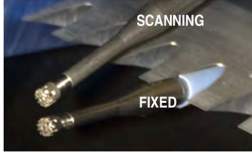
Figure 4.3: Fixed and scanning microphones at their closest spacing of 6 mm, measured from the cartridge centers.
