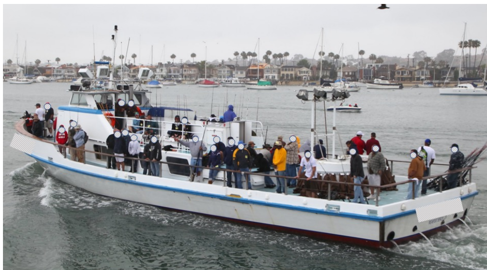
Figure 1.2. Photo of Boat A, a recreational fishing boat equipped with a wet exhaust system that scrubs 100% of all emissions produced by the boat's twin engines and discharges the scrubber washwater and byproducts from the combustion of the fuel being used (in this case, CARB diesel) continuously into the ocean through the outlet holes located on the boat's stern.
