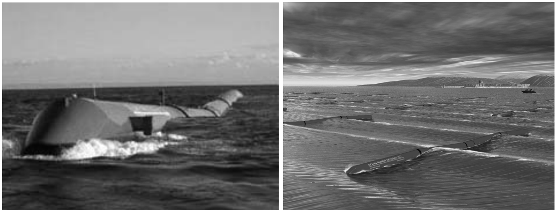
Figure 1.3: Photo of a prototype Pelamis and conceptualized Pelamis wave farm.
