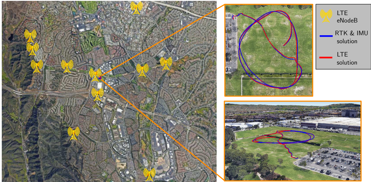
Figure 5.17: Environmental layout of the experiment, location of the eNodeBs, ground truth, and final navigation solution. The UAV traversed a trajectory of 605 m over 175 seconds. The results show a 2-D RMSE of 81 cm. Image: Google Earth.
