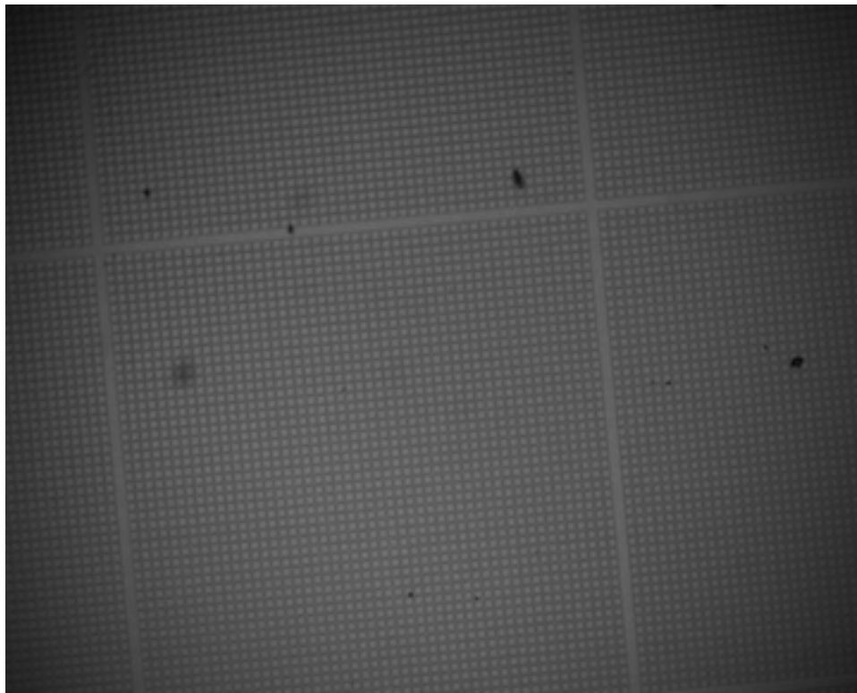
Figure 3-2 Picture of the standard SEM grid used to calibrate the pixel-to-micron conversion factors for each objective lens. The grid consists of 49 \times 49 groupings of 10\ \mu\text{m} \times 10\ \mu\text{m} pitched squares. This picture was taken with our camera using the 20x objective lens.
