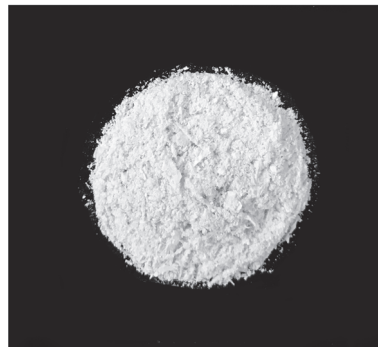
Fig. 2. Dried PHBV samples extracted from H. mediterranei cells. The PHBV polymers were extracted from the cells of H. mediterranei and then washed and dried for storage. The PHBV samples were whitish brittle pieces after oven drying.
