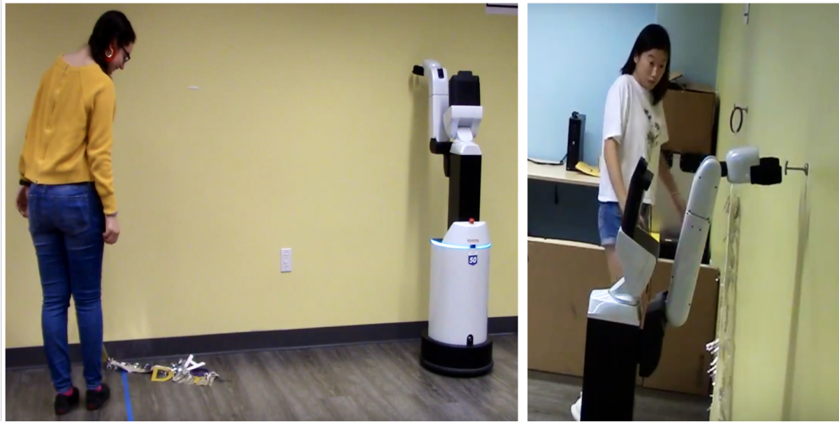
Figure A.2. In our study, a robot and person engaged in proximate, GDJA to collaboratively hang a banner. Intermittently, the robot intentionally dropped the banner 7 cm short of the hook. The robot would still proceed to the “target” location as if it were still trying to hang the banner.
