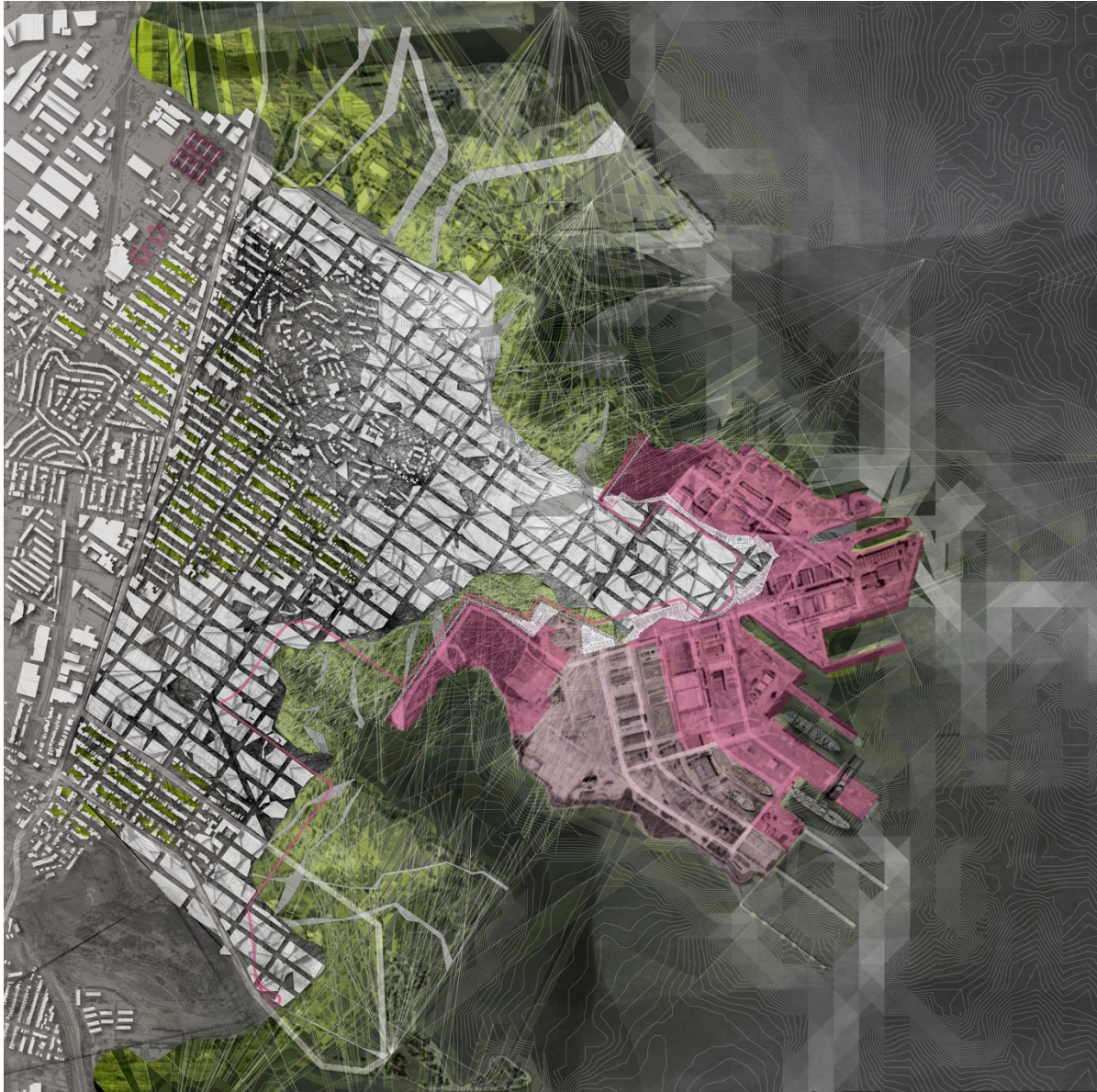
7.10 Urban plan with building blocks constituted as whitespace. The image was created by processing topographic and cultural GIS data through a Grasshopper script in Rhino, followed by post-processing in Illustrator and Photoshop where texture fills were applied. By Kirsten Larson and Cindy Hartono
