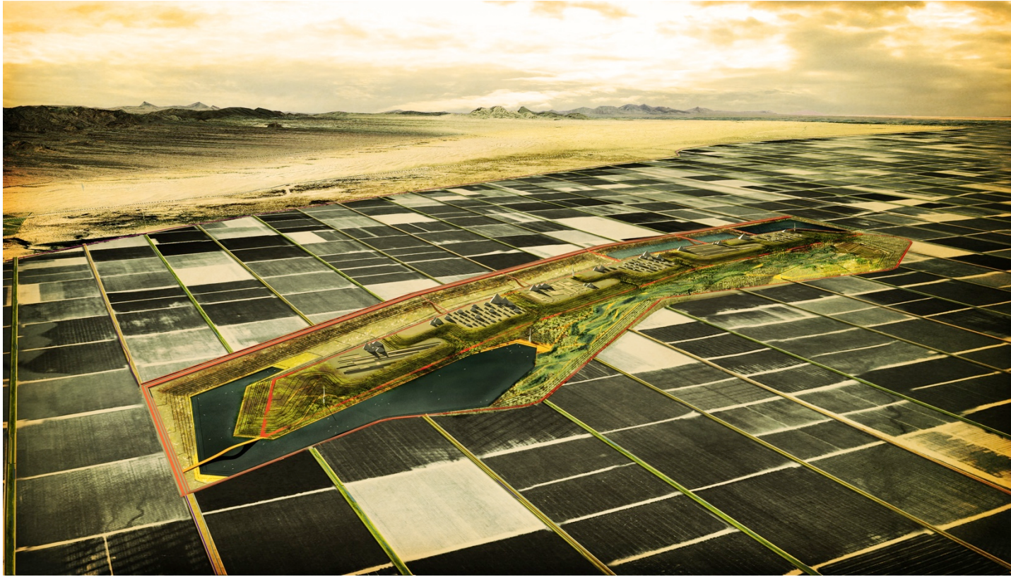
7.12 Bird's eye view that is dramatically illuminated by positioning the sun near the horizon. The image was created by constructing a Rhino 3D model from AutoCAD line-work, view-matching the Rhino view to a scene captured in Google Earth terrain view, rendering in V-ray, and compositing the elements in Photoshop. By Richard Crockett
