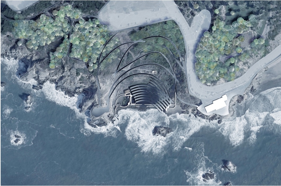
7.4 Design context plan combining watercolor and aerial photography in an image with depth and drama. The image was created by compositing GIS and AutoCAD line-work, aerial photo, and watercolor samples in Photoshop, where color masks were applied, and the contour lines inverted to white. By Yolanta Sui
