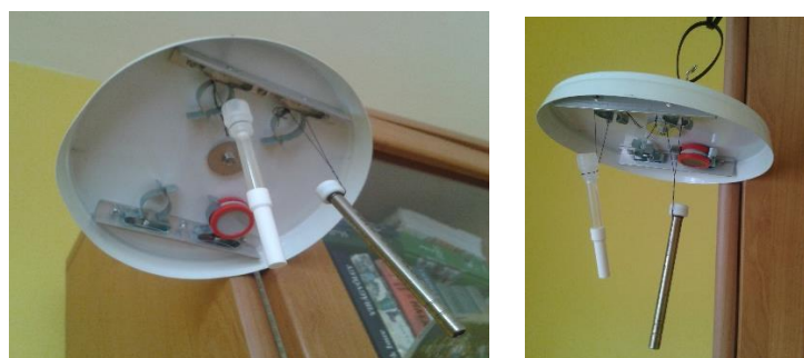
Figure 5.4 Set of passive samplers placed in one living rooms (Source: Author)
