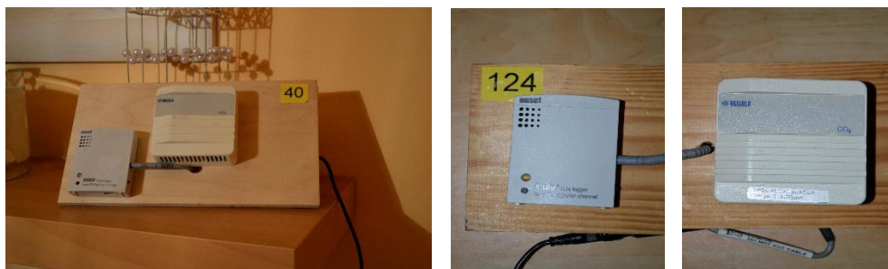
Figure 5.3 HOBO U12-012 and CARBOCAP CO 2 monitors (Source: Author)
