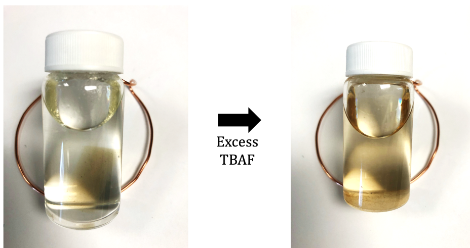
Figure S12. Photographs of swollen HDPE-v before and after the addition of excess TBAF.
