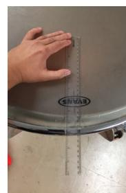
ruler + bow: the five-line staff indicates the bowing positions of the ruler. the top line is furthest away from the timpano; the middle line is the middle point; the bottom line is closest to the timpano. this range is dynamic and relative to the length of the portion of the ruler that is not touching the timpano.
