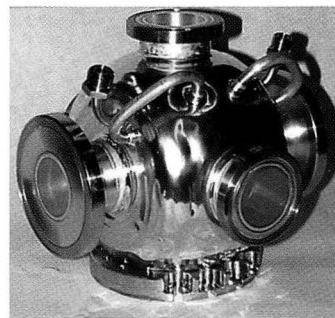
Figure 10. ALS third-harmonic cavity for flattening the rf potential over the length of a bunch, and thus reducing large-angle intrabeam scattering within the bunch.
