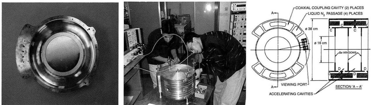
Figure 9. RF cavity (clockwise from top left): internals, schematic, and test preparations.
