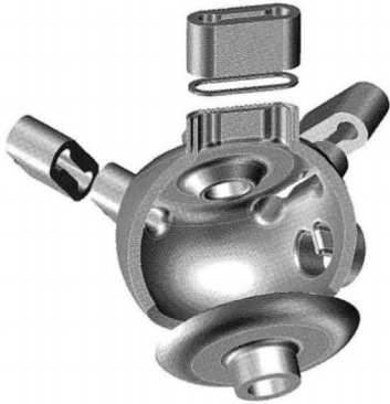
Figure 6. Cutaway of a 714-MHz cavity. The beampipe slants from top to bottom in this view.
