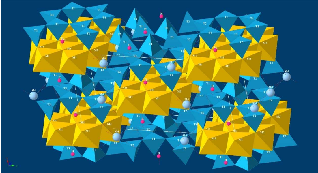
Figure 1.1: The general structure of an amphibole mineral such as tremolite, with monoclinic symmetry crystallizing in the C2/m space group. The x-y-z axes correspond to the a-b-c crystallographic axes
