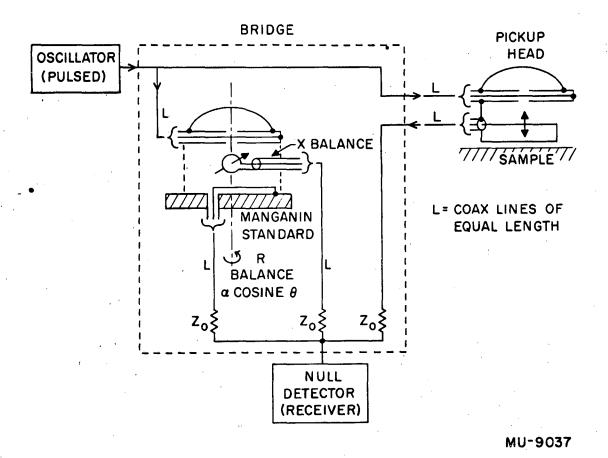
Fig. 4 Manganin standard eddy-current bridge.
