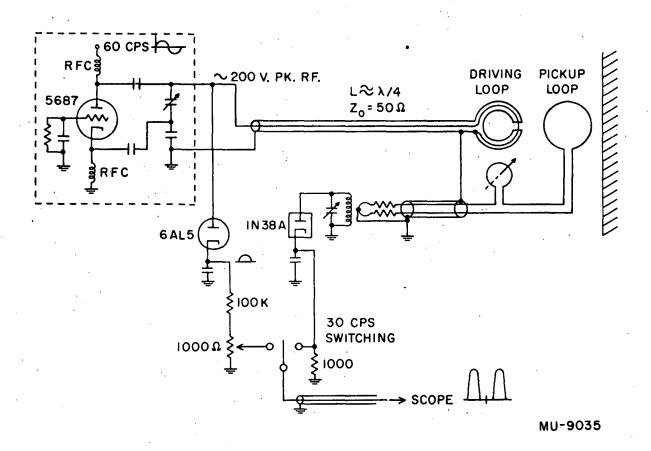
Fig. 1 Circuit diagram of original skin resistance meter.
