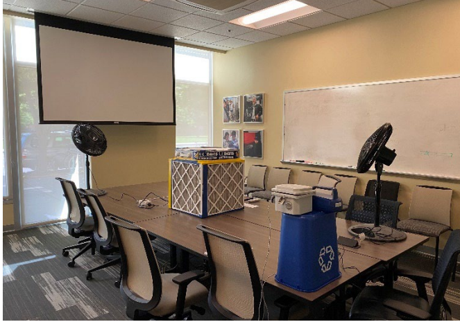
Figure 4-1: CR box experimental test setup in a conference room.
